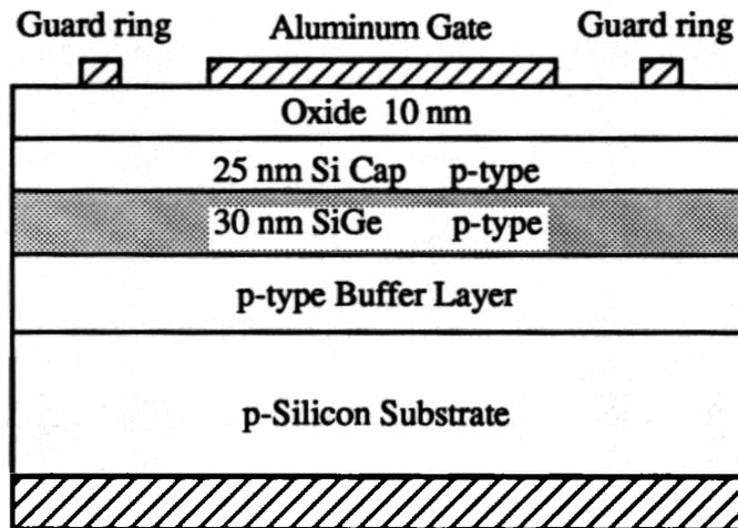
Figure 5.2. Capacitance structure used for testing the generation lifetimes of the  $\text{Si}_{0.82}\text{Ge}_{0.18}$  strained layer. The capacitor is pulsed into deep depletion and monitored during recovery to inversion.
