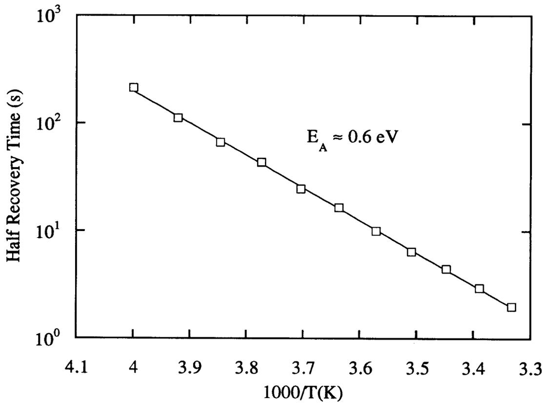
Figure 5.6. Temperature dependence of recovery time for an all-silicon device. The activation energy of this plot is 0.6 eV.
