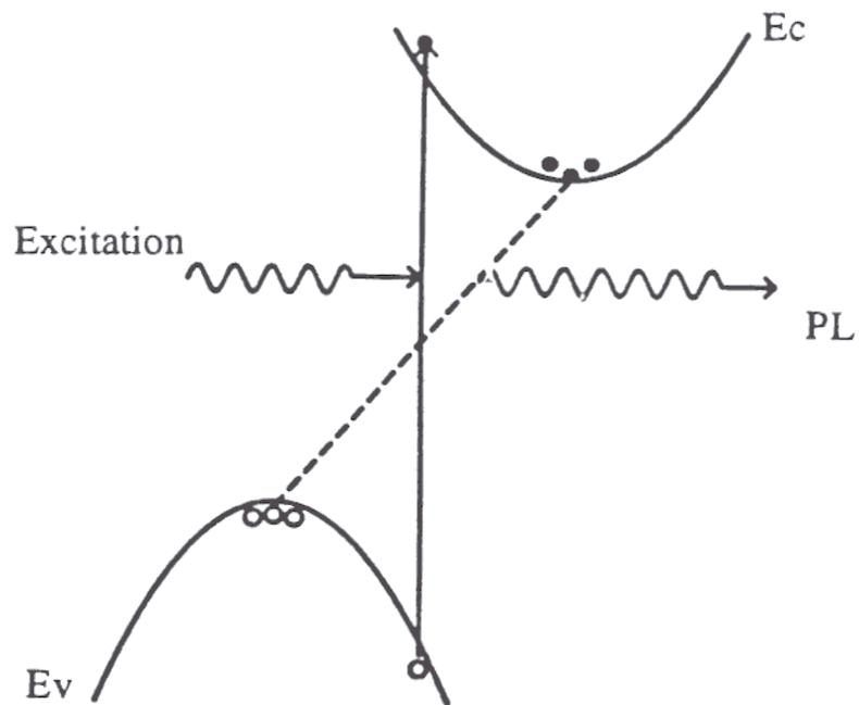
Figure 5.11. Schematic of photoluminescence in an indirect band gap semiconductor. Carriers are excited from the valence band to the conduction band by laser illumination creating an electron-hole pair. The carriers relax to the lowest energy state of the band until they recombine. Phonons or alloy scattering are required to conserve momentum in these materials. Long carrier lifetimes are needed or carriers will non-radiatively recombine at traps.
