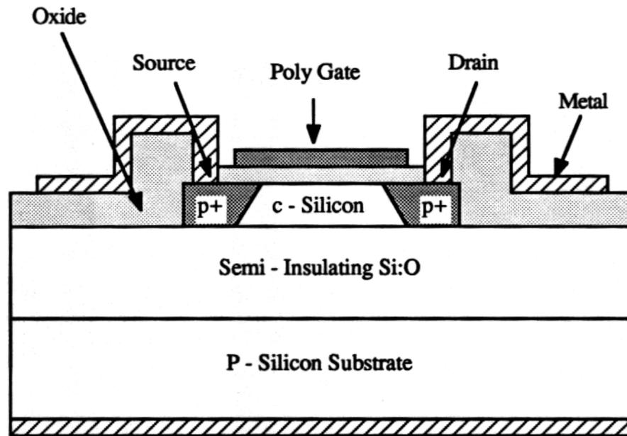
Figure 6.6. Proposed device structure to demonstrate Si:O as a semi-insulating substrate. The oxygen-doped silicon remains crystalline during growth, allowing high quality crystalline silicon (without oxygen) to be grown as the active layer. We fabricated several p-channel and n-channel devices using this structure with gate lengths ranging from 2  $\mu\text{m}$  to 50  $\mu\text{m}$ .
