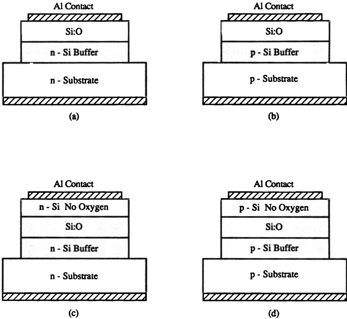
Figure 6.1. Device structures used for testing the electronic characteristics of the oxygen doped silicon layers. (a) Metal - Si:O - n and (b) Metal - Si:O - p were the devices used to measure the resistivity of the Si:O. (c) n - Si:O - n and (d) p - Si:O - p were used to determine the carrier mobilities.
