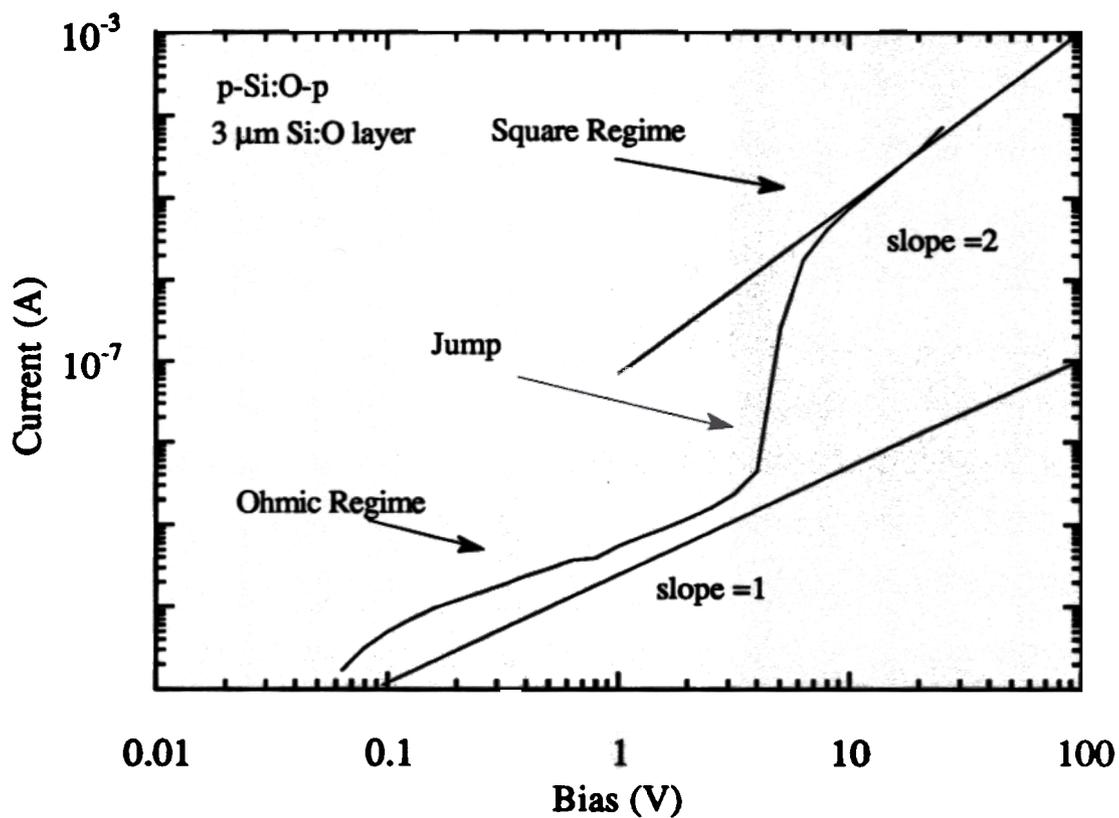
Figure 6.5. Current vs. Voltage for a p-i-p structure with a silicon layer doped to  $2 \times 10^{20} \text{ cm}^{-3}$ , with oxygen doped layer forming the intrinsic region. Notice the three regimes; Ohm's Law, "jump" corresponding to trap filling, and square law due to space-charge. The jump indicates a single trap level within the band gap.
