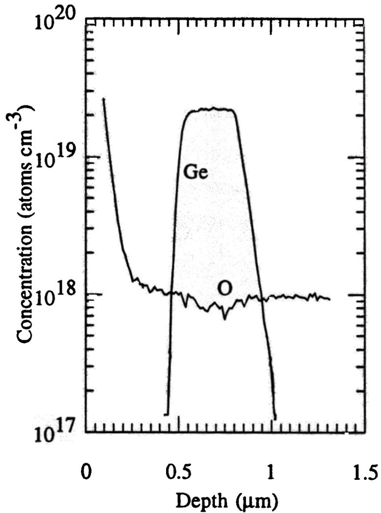
Figure 4.3. SIMS plot of silicon-germanium grown at 625 °C with little oxygen contamination. The oxygen concentration is below the detection limit of SIMS. This sample was grown after the load-lock was installed on the system. The load-locks prevents oxygen and water vapor from contaminating the chamber between depositions.
