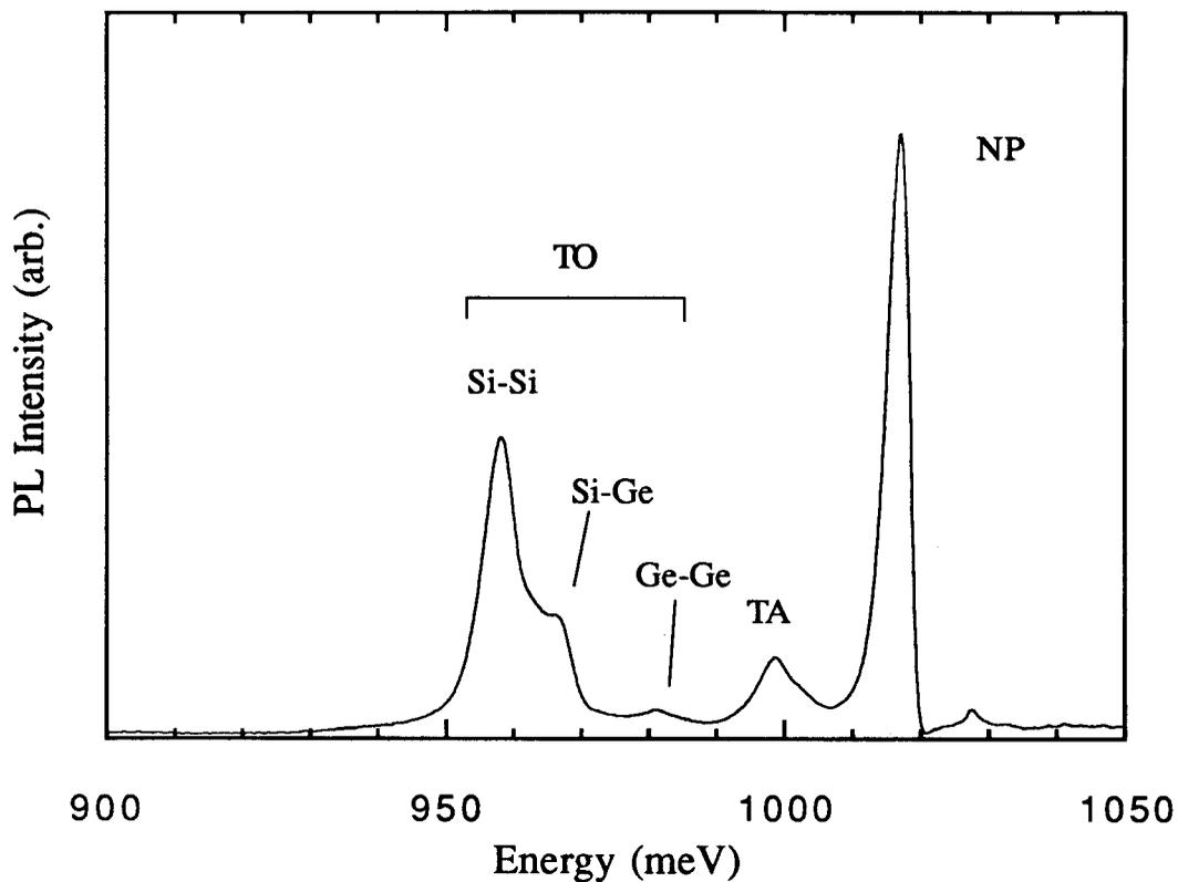
Figure 5.12. 4K Photoluminescence spectrum of a 30 Å thick  $\text{Si}_{0.80}\text{Ge}_{0.20}$  strained layer. The no-phonon (NP) line is due to the randomness of the silicon-germanium alloy and occurs just below the band-edge of the silicon-germanium. The phonon replicas are clearly visible and correspond to the different chemical bonds in the material, Si-Si, Ge-Ge, and Si-Ge. The luminescence is due to bound excitons.
