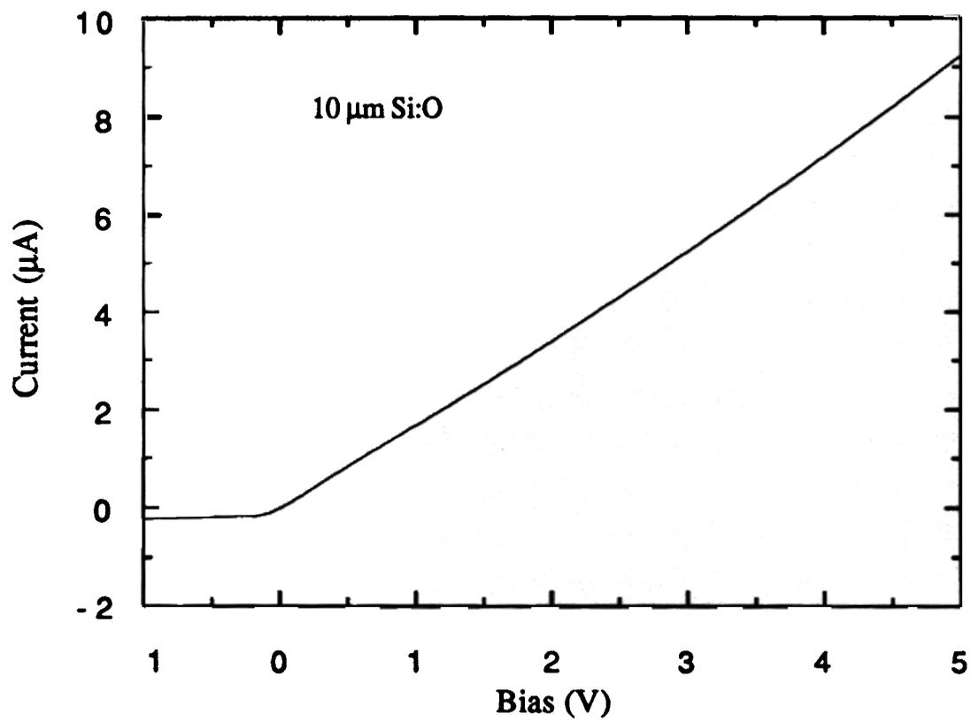
Figure 6.2. Room-temperature Current-Voltage characteristics of the metal - (Si:O) - (n-Si) device. Note that the full-scale current is only 10  $\mu\text{A}$  for a 50 V bias. This demonstrates the high resistivity of the oxygen-doped silicon. The device area is  $1.8 \times 10^{-3} \text{ cm}^2$ .
