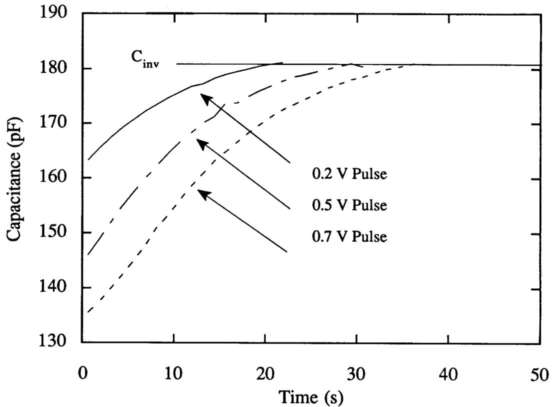
Figure 5.3. Capacitance recovery vs. time. Three different voltage pulses were applied to this capacitor, 0- 0.2 V, 0 - 0.5 V, 0 - 0.7 V, and the capacitance was recorded with time. The capacitors recover from deep-depletion to inversion ( $C_{inv}$  is shown on the plot). Notice that the recovery times increase with increased voltage pulse.
