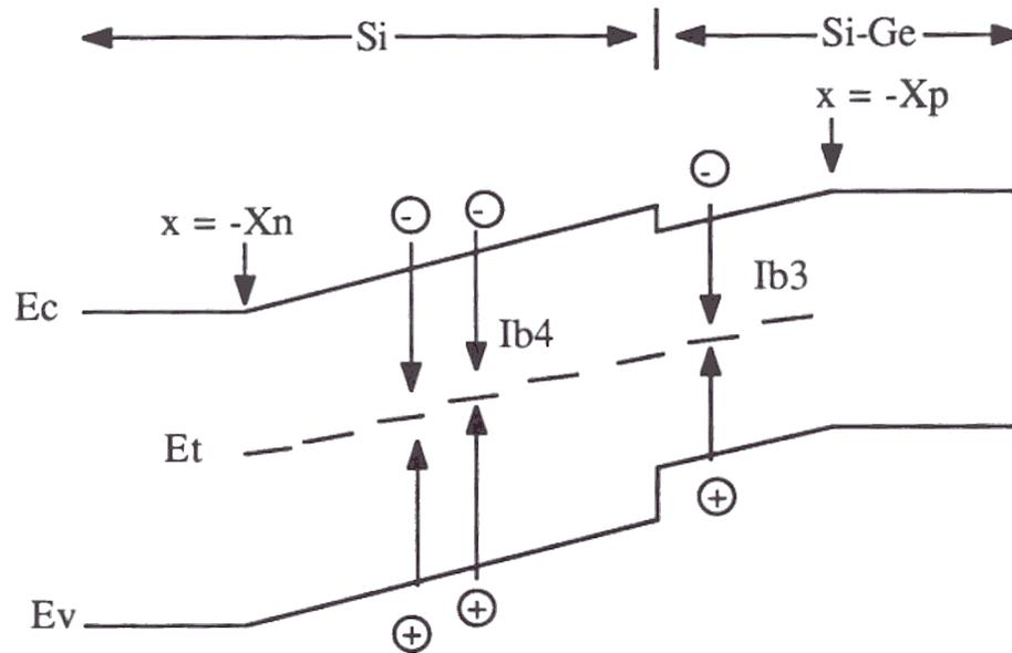
Figure AI.1. Expanded view of recombination in the space charge region.  $I_{b4}$  is the recombination in the lightly doped emitter side of the junction while  $I_{b3}$  is due to recombination in the depletion region on the heavily-doped, narrow-gap side of the junction. For  $I_{b3}$  to dominate, the lifetime in the heavily doped material must be much shorter than the lifetime in the lightly doped material. This condition yield an "n=1" base current.
