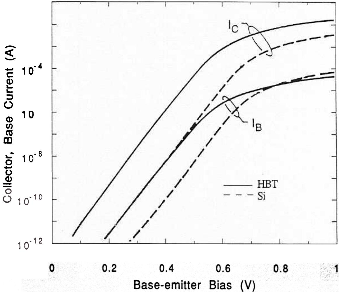
Figure 5.9. Gummel plot of a Stanford HBT (King). The plot of the logarithm of the base and collector currents as a function of base-emitter bias. The HBT exhibits the expected increase in collector current as expected, but the base current of the HBT has also increased which was not expected. The ideal slopes of the base current coupled with the increased base current suggest that the device is limited by recombination of carriers in the base region.
