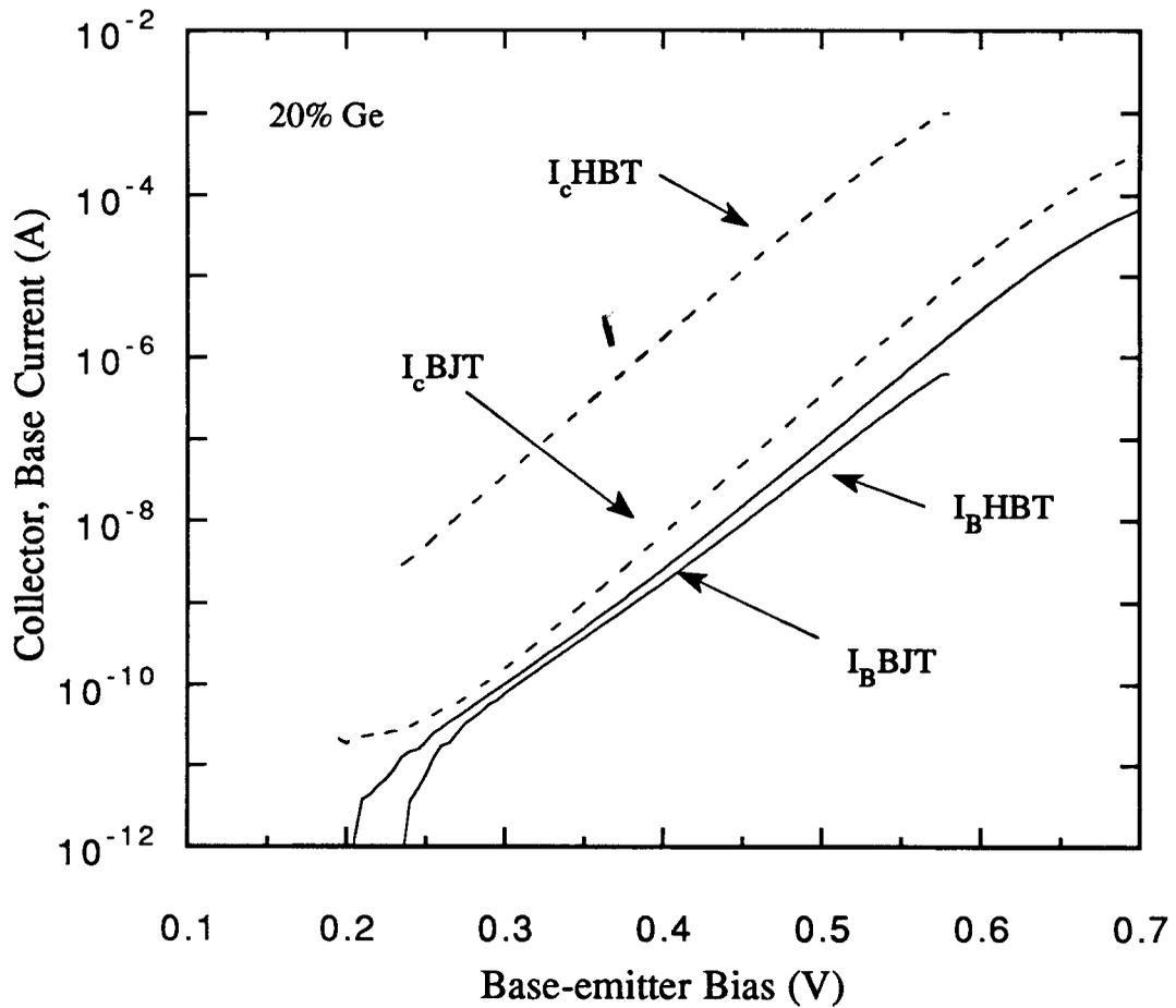
Figure 5.10. Gummel plot of a Princeton University HBT. The oxygen concentration in the base region of these devices was below the detection limit of SIMS ( $<10^{18} \text{ cm}^{-3}$ ). The HBT has the enhanced collector current over the homojunction device as expected and has no increase in base current as expected. This HBT is an injection limited device, neutral base recombination is not the dominant source of base current.
