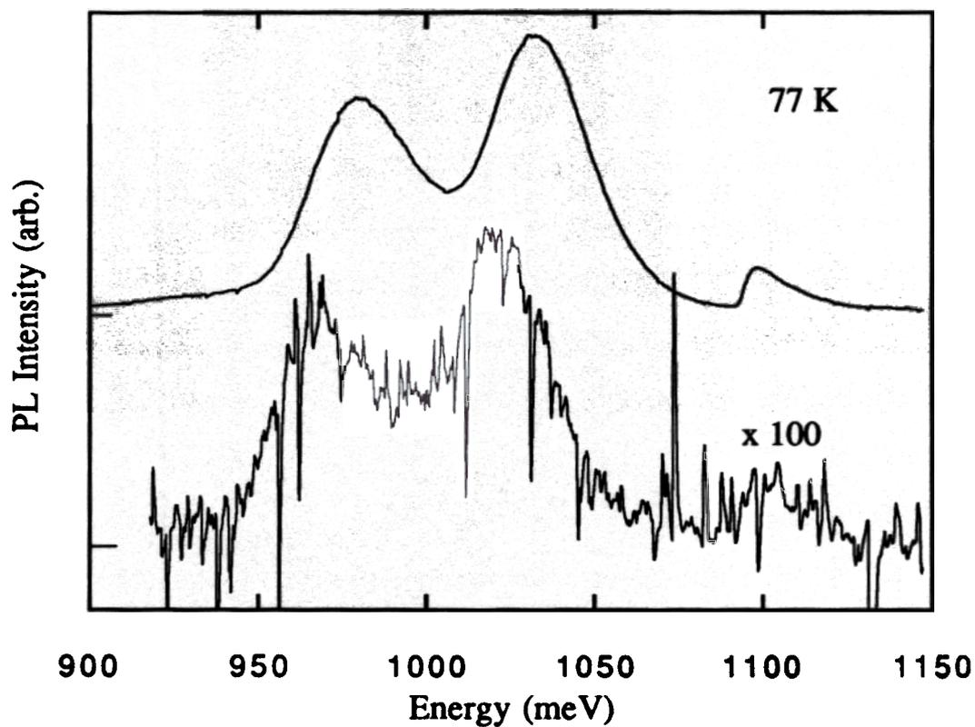
Figure 5.13. PL spectra of silicon-germanium layers grown in a well baked system and a newly vented system. The top spectrum corresponds to a silicon-germanium sample grown in a baked-out system and the bottom spectrum corresponds to a silicon-germanium layer grown as the second sample after the system was vented. Notice the factor of 100 difference between the two scales. The luminescence is due to free excitons.
