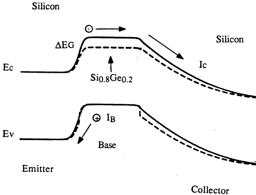
Figure 5.7. Band diagram for a heterojunction bipolar transistor and a silicon homojunction device. The the base region of the HBT has a narrower band gap which leads to a lowering of the conduction band in the HBT compared to the BJT. This lowering of the conduction band increases the gain of the device. Also shown are the collector current and the base current.
