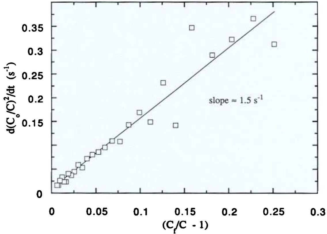
Figure 5.5. Zerbst plot of a recovering capacitor. The Zerbst analysis is effectively plotting the generation volume vs. the generation rate and extracting a lifetime from the slope. The lifetime is directly proportional to  $n_i$  and inversely proportional to the slope of the Zerbst plot. The lifetime of this capacitor is  $\sim 2 \mu\text{s}$ .
