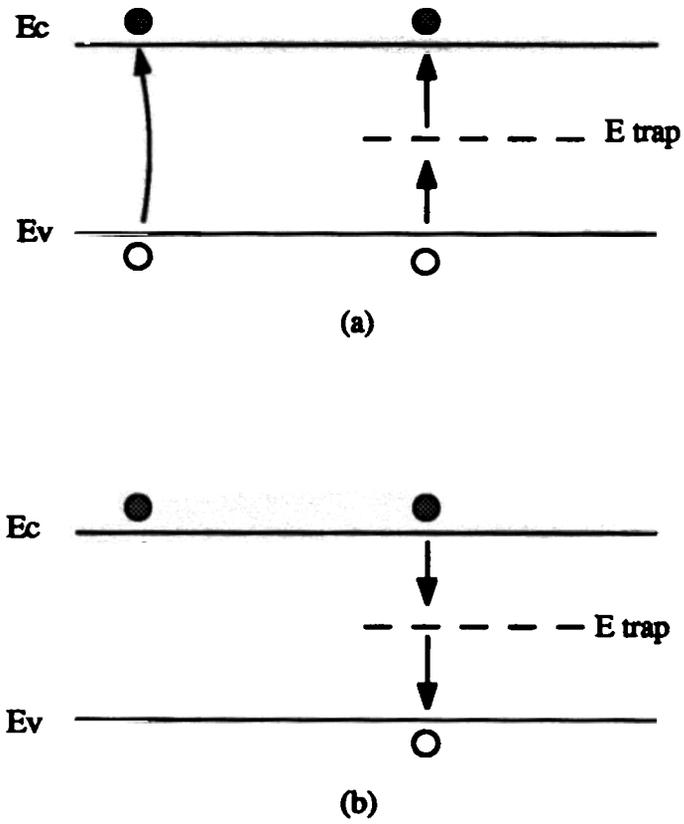
Figure 5.1. Schematic diagrams of carrier (a) generation and (b) recombination. Both processes can occur directly across the band gap or indirectly through mid-gap traps. In indirect band gap materials such as silicon and silicon-germanium, direct recombination and generation are slow and mid-gap states are needed to speed the recovery.
